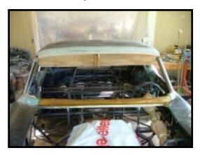
Shown below: Foam and fiberglass are used to build out the pillars between the windshield and side window. Body work along the windshield bottom has been roughed in with body filler.
