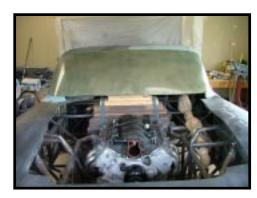
To support the weight of the windshield glass, I built a metal support under the cowl area from 3/4" square tubing. It took a few hours of bending, checking fit, and then more bending to get the proper fit. When it was good enough it was welded in place and vertical supports added for strength. This cowl support then became the platform for more foam and fiberglass to go along the windshield bottom.
