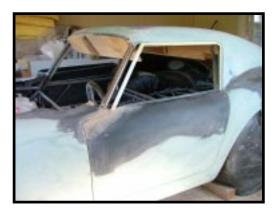
stack of wooden blocks and shims to achieve to proper height. To hold the top in place, I drilled holes in the fiberglass windshield and used wood screws to secure it to a plywood form behind it. Drilling holes and securing with screws is certainly not an option if you're dealing with real glass. The section of the roof that mates to the windshield was then formed so it matched up to the shape of the windshield.
