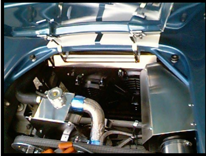
Shown above: The final result from revamping the cooling system came out nice. New is a fan mounting frame covered by a stainless steel shroud, a temperature adjustable fan switch, and a degas/surge coolant tank.
